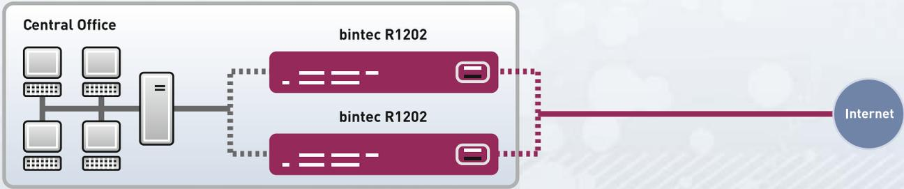
**Device redundancy through BRRP:**
